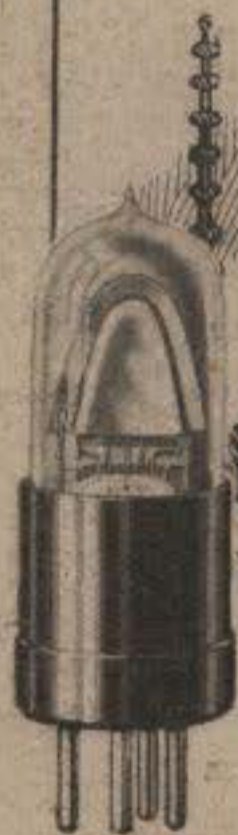
Cossor W.3 Loud Speaker Valve Filament Volts - 1.8 Consumption - 5 amps. Price 18/6
